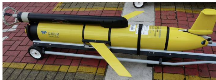
Figure 3.1: Slocum G2 underwater glider with Ocean Microstructure.
