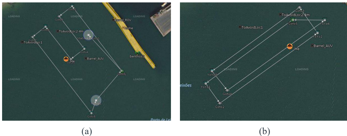
Figure 4.3: Neptus mission plans for the mapping (a) and profiling (b) runs.
